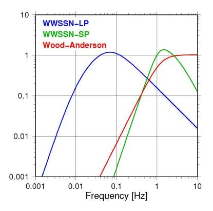
**Figure 1.** Displacement amplitude-frequency responses of the classical seismographs: WWSSN-SP, WWSSN-LP and Wood-Anderson (WA), normalized at the frequencies  $(f_n)$  in the caption of Table 1.
