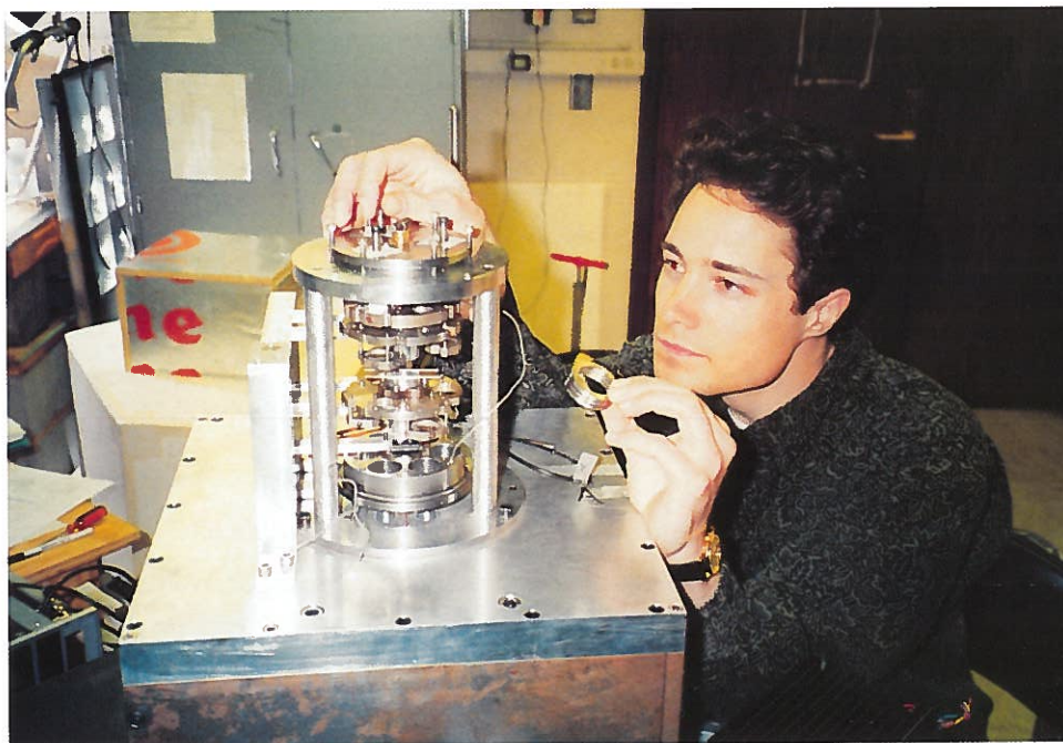
Laboratory measurements of wave attenuation in mantle-like materials and the resulting velocity dispersion at seismic frequencies (0.001 to 10 Hz) are essential for interpreting seismic wave data in terms of the composition and properties of the interior of the Earth. (Courtesy Hartmut Spetzler, Rock Physics Laboratory, University of Colorado.)
